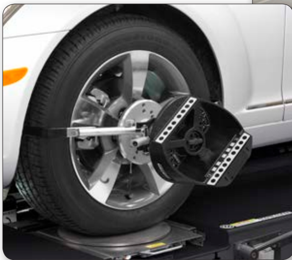
Targets contain no electronics to damage if dropped.
