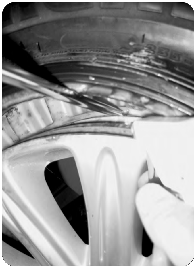
Generously apply lubricant between support ring and wheel. Allow lubricant time to work.
