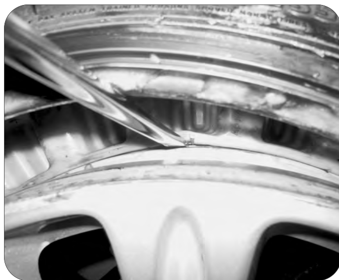
Pull support ring slightly away from wheel for lubrication.
