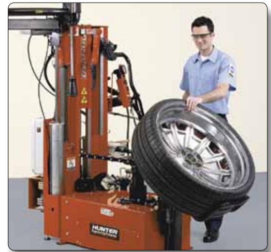
Match-mounting the stiffest point on a tire to the low spot on a rim makes the assembly roll as round as possible.
