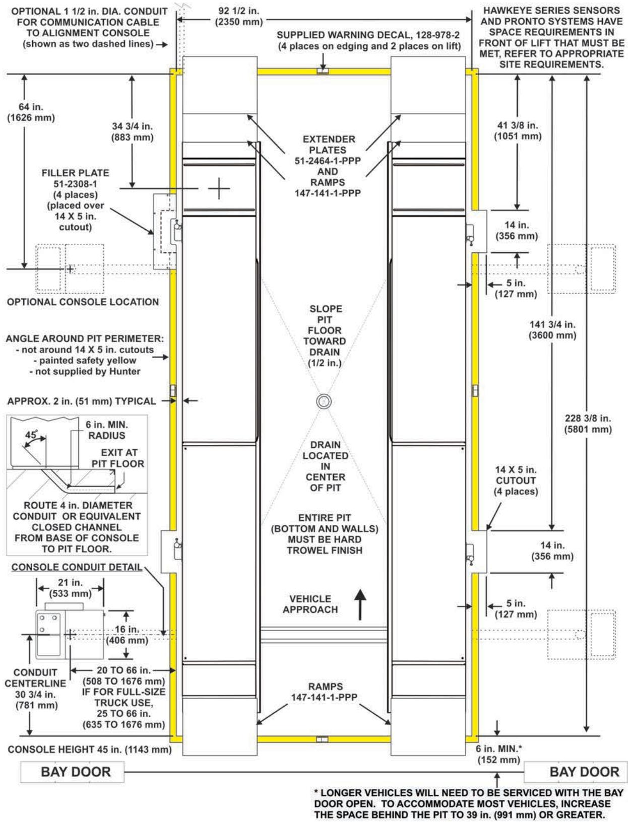
Dimensions shown are for end result. Tile thickness (if applicable) must be considered before pouring concrete. Positioning of control console is limited to a maximum space between console and rack of 5 1/2 feet (1676 mm) at the approach ramp end and 16 feet (4877 mm) at the turnplate end.
