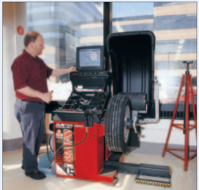
Time Study Garage engineers also develop service standards using Hunter vibration management technology.
