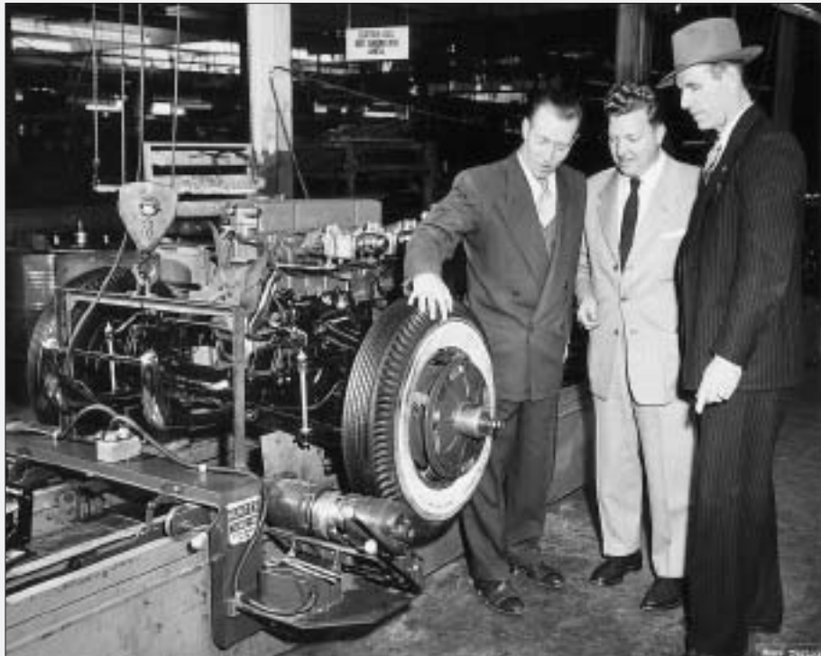
Hunter and Chevrolet managers with the Hunter Tune-In wheel balancer mounted on the front wheel of this partially assembled 1954 Corvette.
