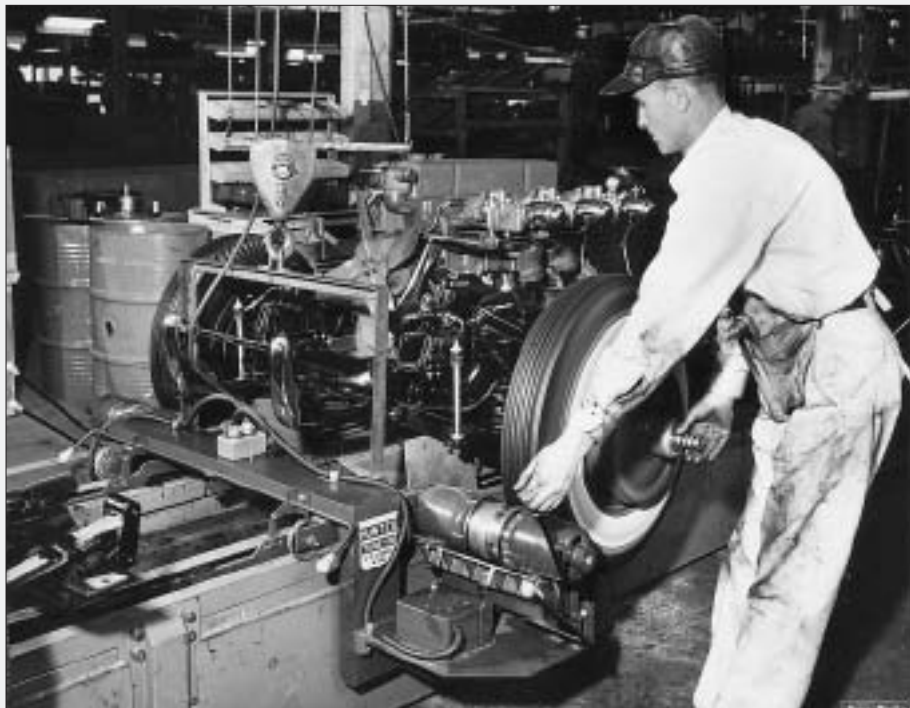
With the mounted wheel spinning, the technician adjusted knobs on the Tune-In to balance the wheel. Weights were then placed where indicated by the balancer.
