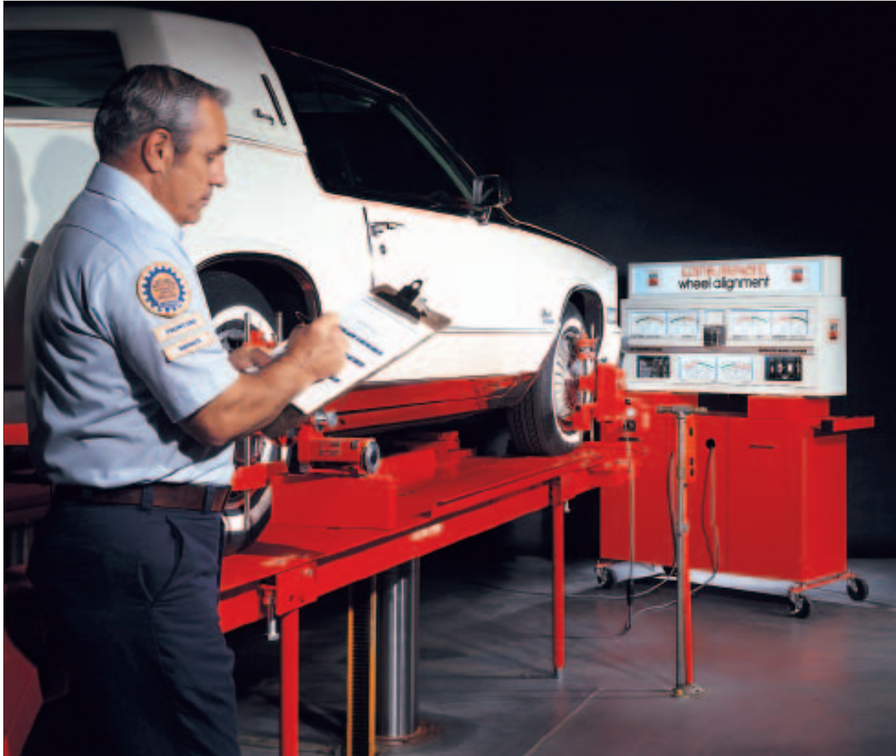
The Hunter S7M-TA Electron-A-Line computerized alignment system shown here featured a mobile cabinet and four electronic, wheel-mounted sensors for four-wheel "Total Alignment" capability. Cabinet options also included stationary and rail-mounted models.
