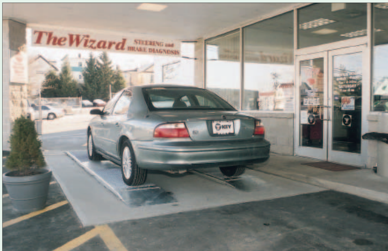
Arriving vehicles have brakes and wheel sideslip tested on the Hunter B400 Brake Tester and SS100 Sideslip Meter. A flat screen monitor mounted in the service area window guides the driver. Customers see the results on the system console located at the write-up counter inside.
