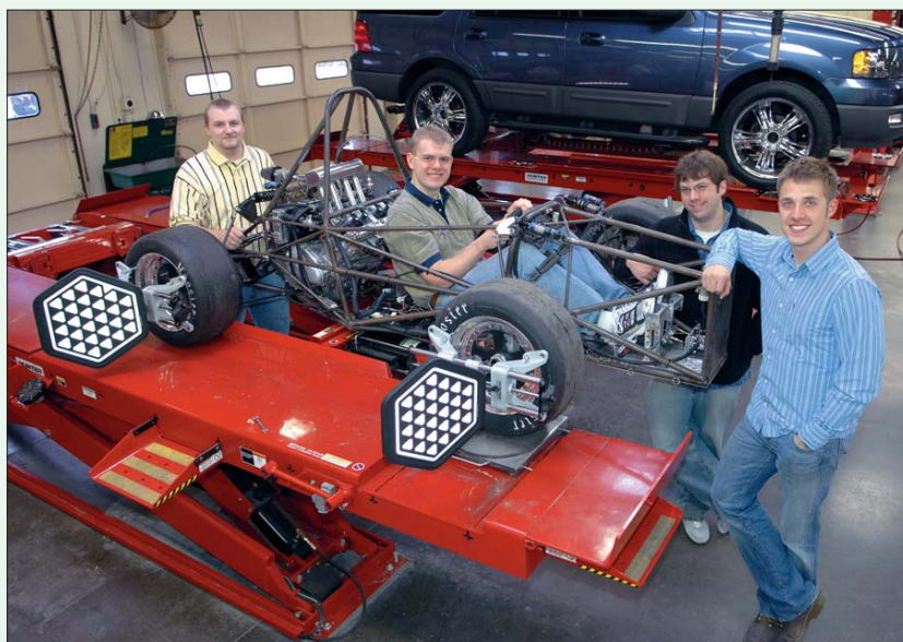
Washington University engineering students Ryan Hyslop, Jake Sparks, Joe Nelson and Eric Jensen measure alignment and frame angles of their Formula SAE car at Hunter's Research & Training Center in St. Louis.
