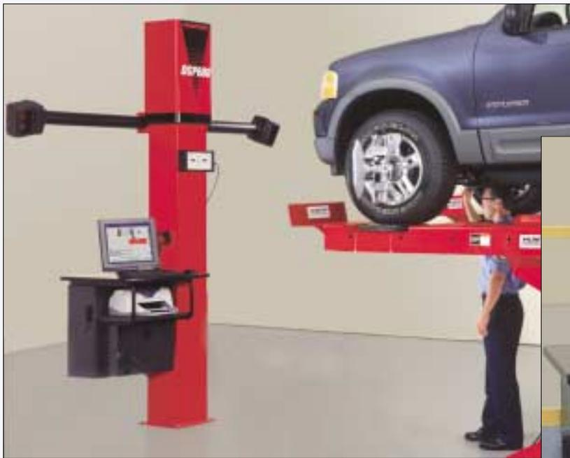
*The W811P-Plus Aligner is shown mounted to an optional DSP600 Sensor tower (left) and an optional pit wall (below).*
