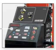
**FIA** console Controls PowerSlide and Inflation Station features.
