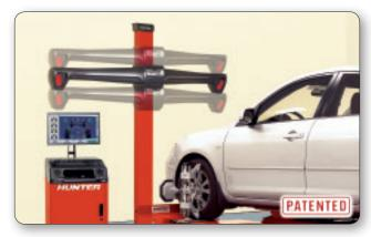
Lift-column configurations automatically position the cameras to any lift height during the alignment process.
