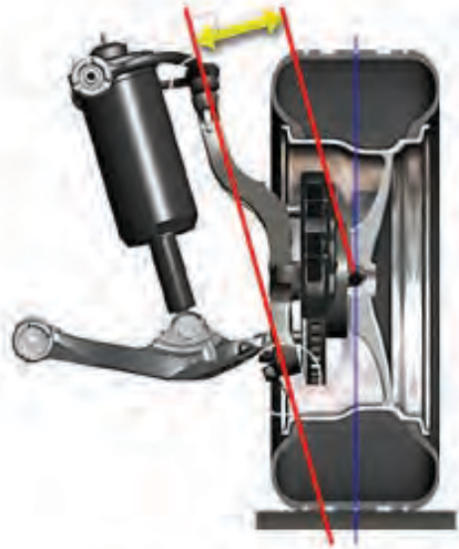
Figure 831 - Positive Rolling Force Lever - Right Side
