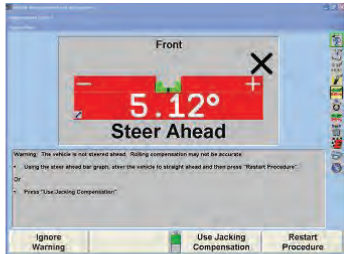
Figure 76 - The vehicle is not steered ahead.
