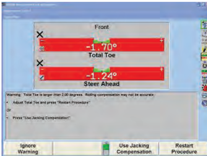
Figure 77 - Total Toe is larger than the preset tolerances.
