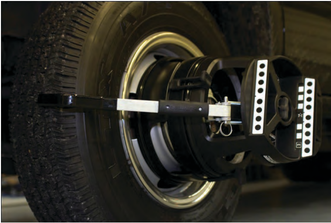
Figure 52 - Mounted on front axle of dually truck wheel
