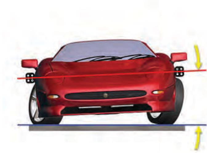
Figure 827 - Positive Body Roll Angle
