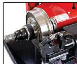
... set up drum service assembly and extend drum boring bar.
