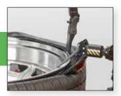
Thin, broad head alleviates stress on bead, and is durable enough to withstand immense mounting forces.
