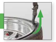
Tool head inserts into tyre, pulls bead over and demounts in one fluid down/up motion.
