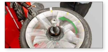
The Auto34R's bead rollers allow spinning of tyre on rim, helping match-mount stiffest point on tyre to low spot on rim.
