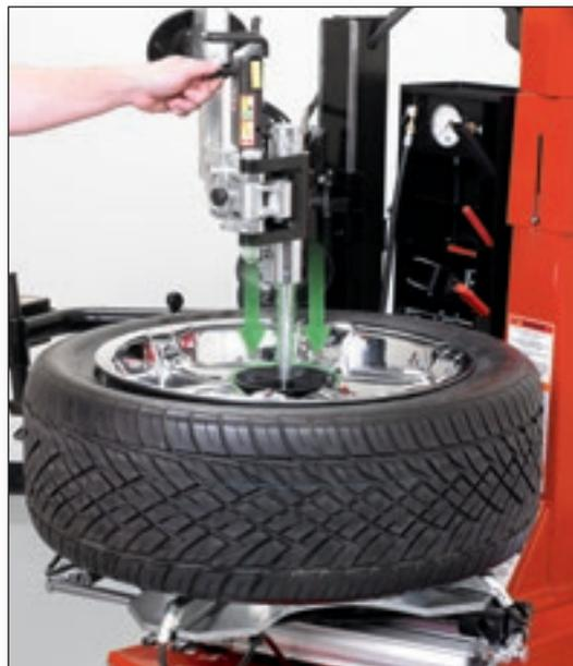
Wheel press cones and extension arm simplify external clamping when servicing low-profile tires.
