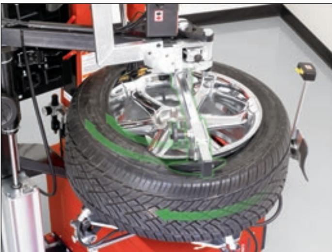
A single bead press roller disc with rotating arm can quickly mount and demount stiff sidewall tires.
