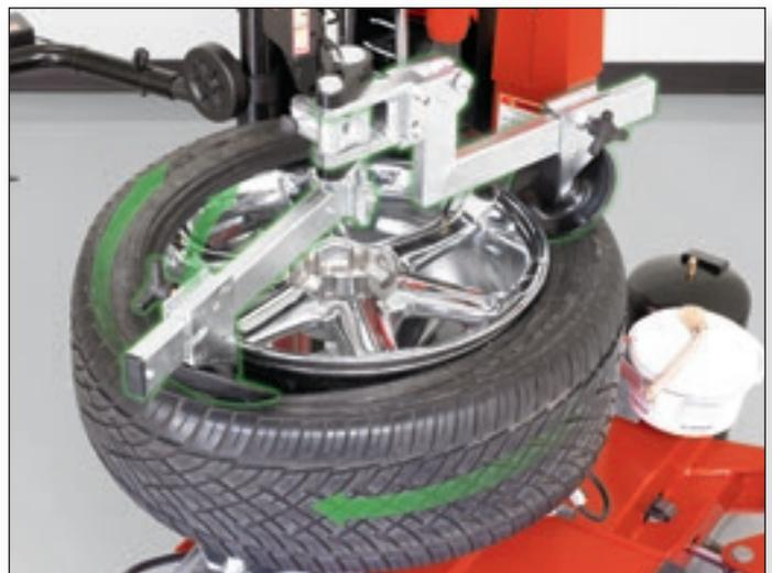
The flip down, fixed bead press arm adds additional contact to service the most extreme low-profile tires and deep drop-center wheels.
