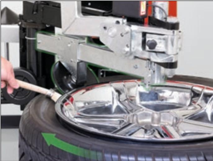
Tapered roller discs assist bead lubrication and ease demounting.
