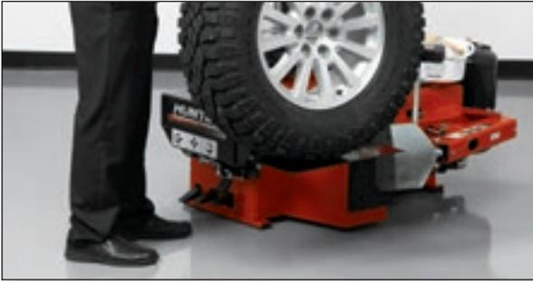
Optional wheel lift eases servicing of large assemblies. Allows for more careful handling of expensive wheels. (20-2045-1)
