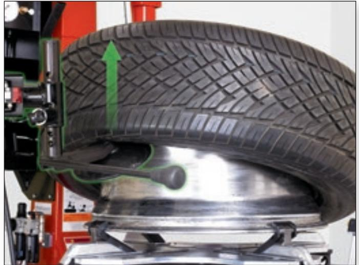
The bottom roller disc can be used for bottom bead re loosening, demounting or match mounting.
