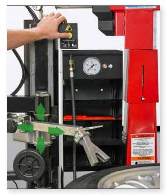
Large tank provides ample volume to seat the toughest tyres. Simply set the position, select inflation mode then press the inflation pedal.
