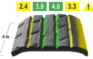
Accurate tread depth calculated for each groove.
