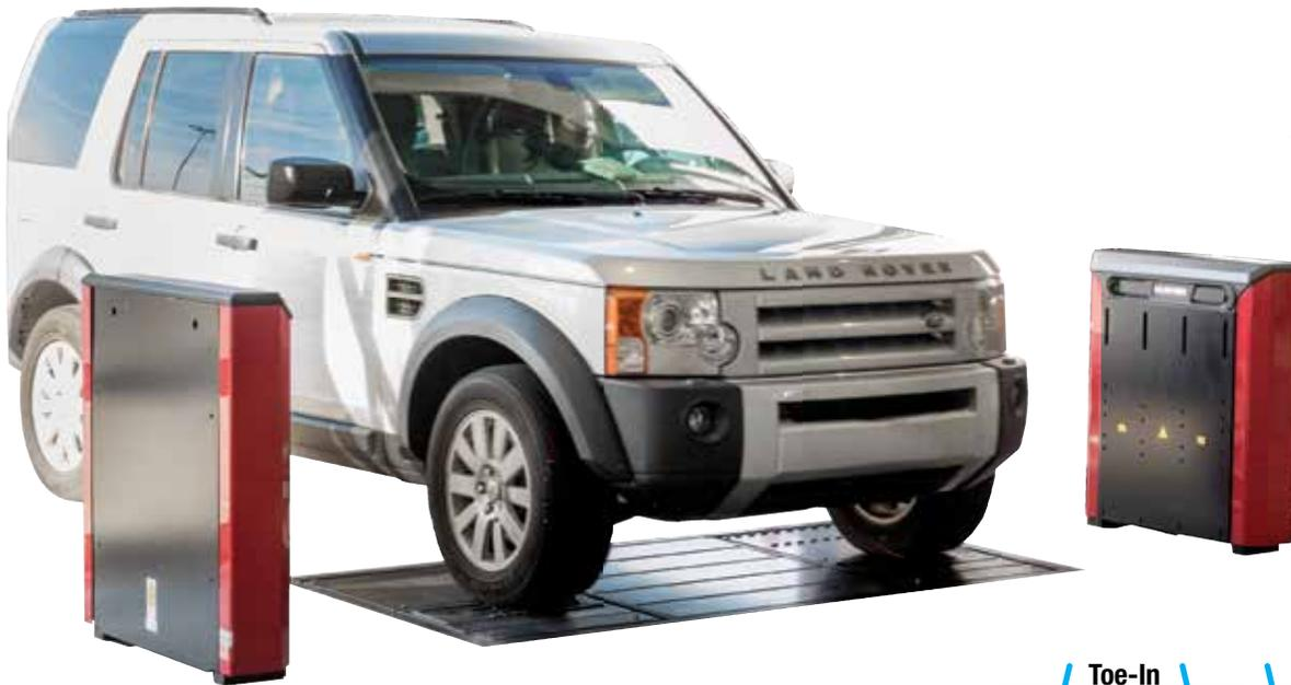
**Quick Check Drive®** automatically measures individual camber and total toe.
