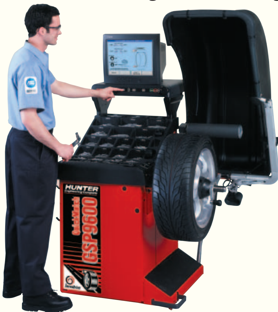
The GSP9600 load roller places up to 300 lbs. of force against the wheel assembly as it turns.
