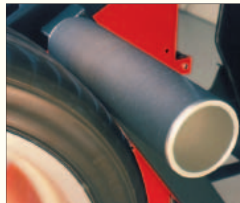
The GSP9600 load roller places up to 300 lbs. of force against the wheel assembly as it turns.
