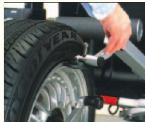
Dataset® Arms improve the accuracy and speed of data entry and weight placement, and measure lateral and radial rim runout.
