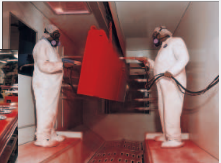
While most of the powder application is automated, production staff monitor quality and even out the application where necessary. An electrostatic charge attracts the powder to the part surface prior to the oven gelling process.
