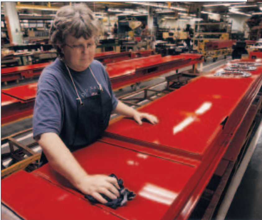
Finished alignment rack runways are ready for assembly. With its unique combination of extreme durability and high-quality appearance, powder coat finish has quickly become a favorite for many automotive industry applications.
