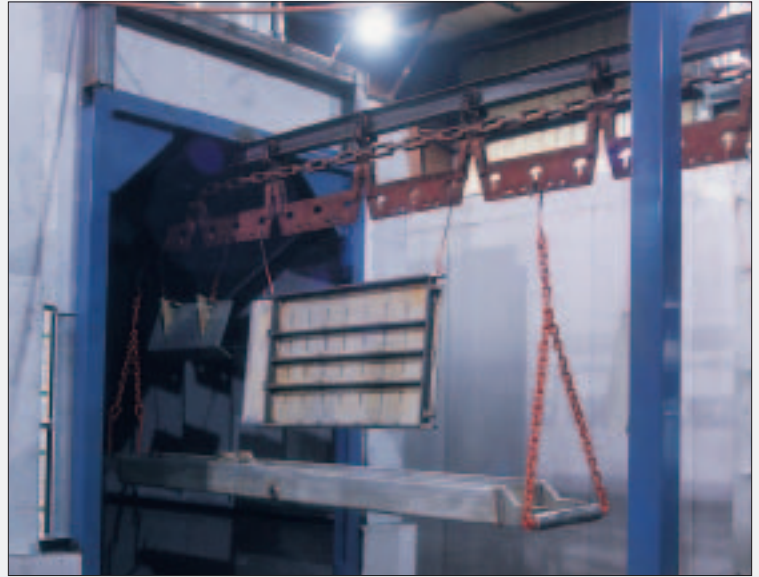
In a highly automated process parts receive a phosphate wash and are dried in ovens prior to application of the resin powder.
