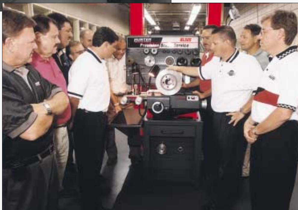
Class members review new HunterPro™ Lathe Packages after cutting brake rotors on this BL505 Bench Brake Lathe.
