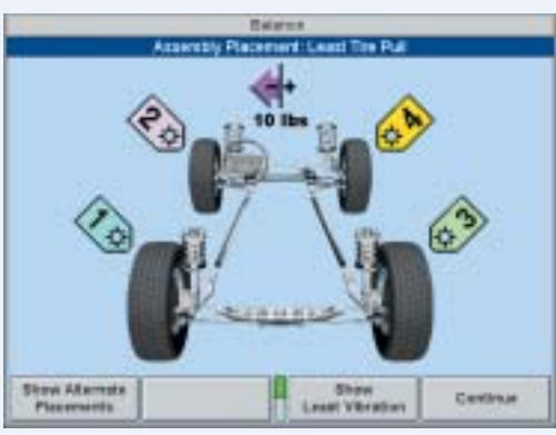
The GSP9700 software suggests tire placement to minimize or eliminate tire-related drift and pull.
