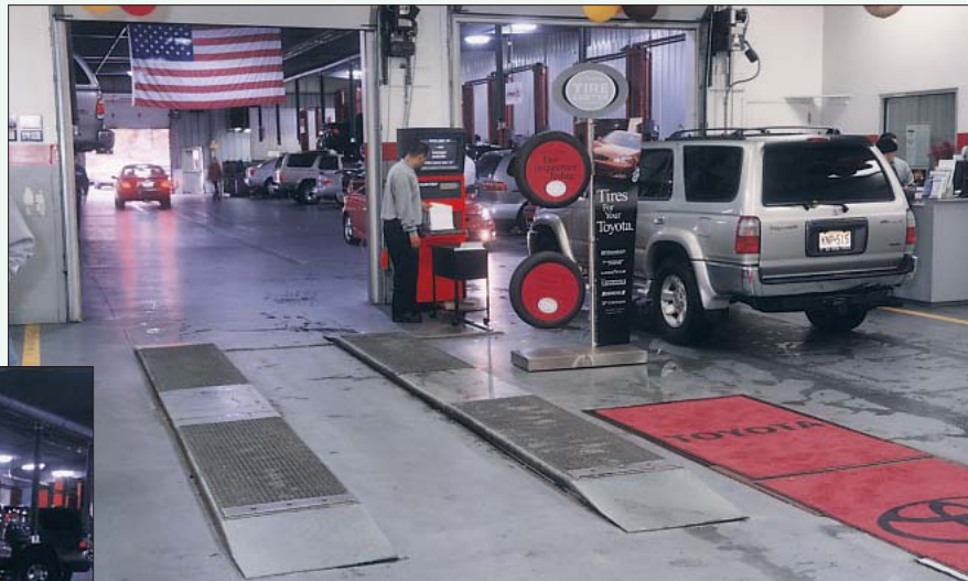
The B400 brake test plates and console are located at the entrance to the dealership's service areas allowing brake testing during check-in.
