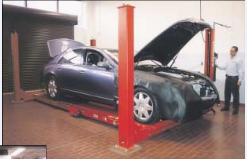
One of three Hunter four-post MKS-MB alignment lift racks in Mercedes-Benz USA's Montvale, New Jersey, Training Center. Montvale is one of the two Hunter-equipped Mercedes-Benz Maybach training facilities in the U.S.
