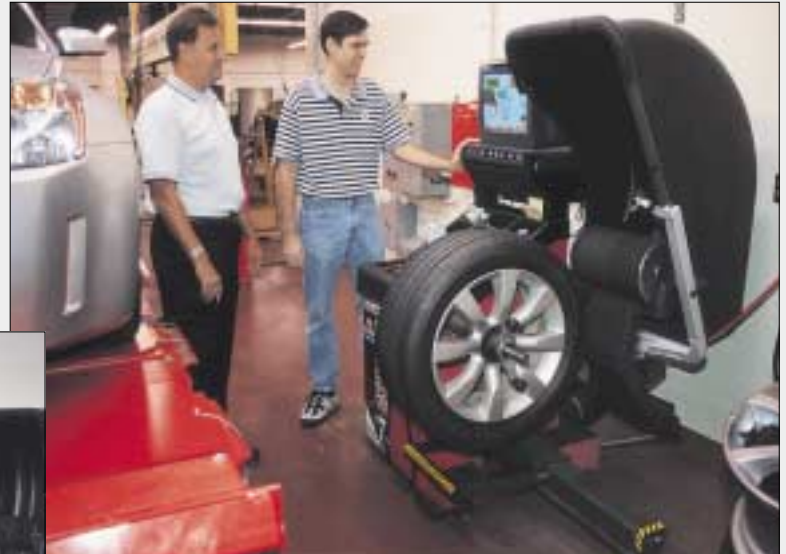
Nissan engineering staff David Shaw, left, and Jeff Gratias use the GSP9700 StraightTrak® feature to measure for any tire pull characteristics in this Nissan performance wheel. The GSP9700 also plays a role in Nissan's Chassis Systems Engineering.
