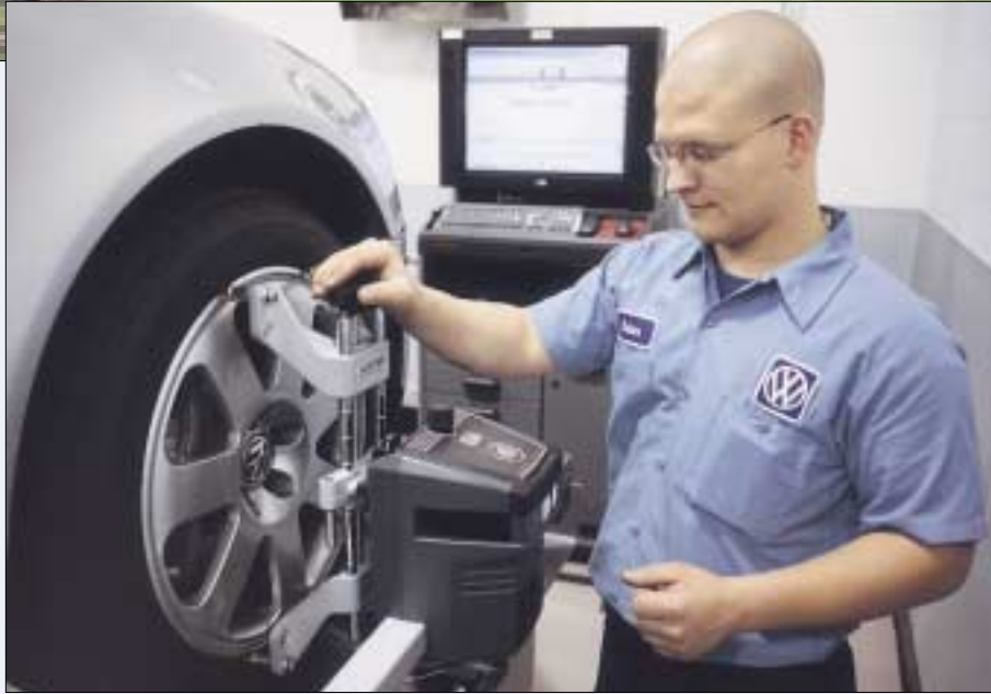
This Volkswagen technician sets up an alignment procedure on a new Phaeton model in V.A.G's U.S. Headquarters service engineering garage.
