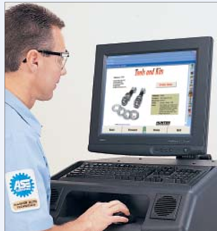
Tools & Kits "Order Now" feature of WinAlign® Software 7.0 lets technicians order parts online from the aligner console.
